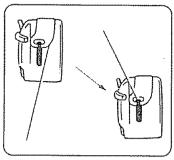
Pull thread under tension Holding latch open, position Case should lock into place spring and through the opening as shown above.
